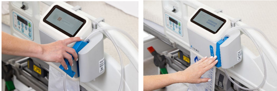
Figure 10 – FIZE kUO Disposable Kit insertion to console
